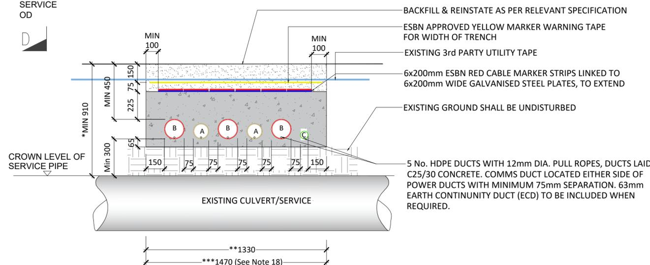
\* ALL EXISTING SERVICES WITH COVERS LESS THAN MIN. DIMENSIONS ABOVE SHALL BE CROSSED BY UNDERCROSSING METHOD
